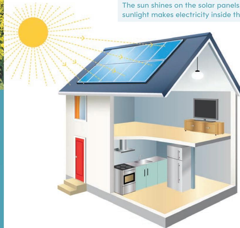
The sun shines on the solar panels, and the sunlight makes electricity inside the panels.
